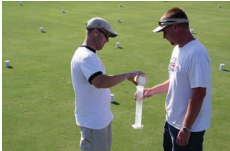
Figure 4. University of Florida graduate students Nick Pressler (left) and Mark Mitchell use a graduated cylinder to measure catch-container collection volumes on a golf green.
