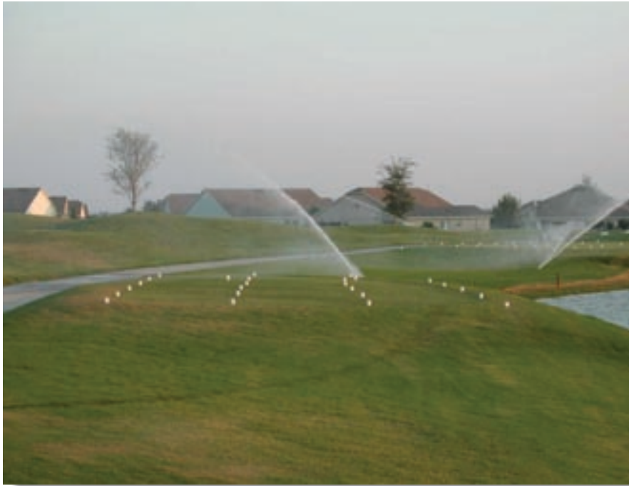
Figure 3. A catch-container test is set up on a tee area.
