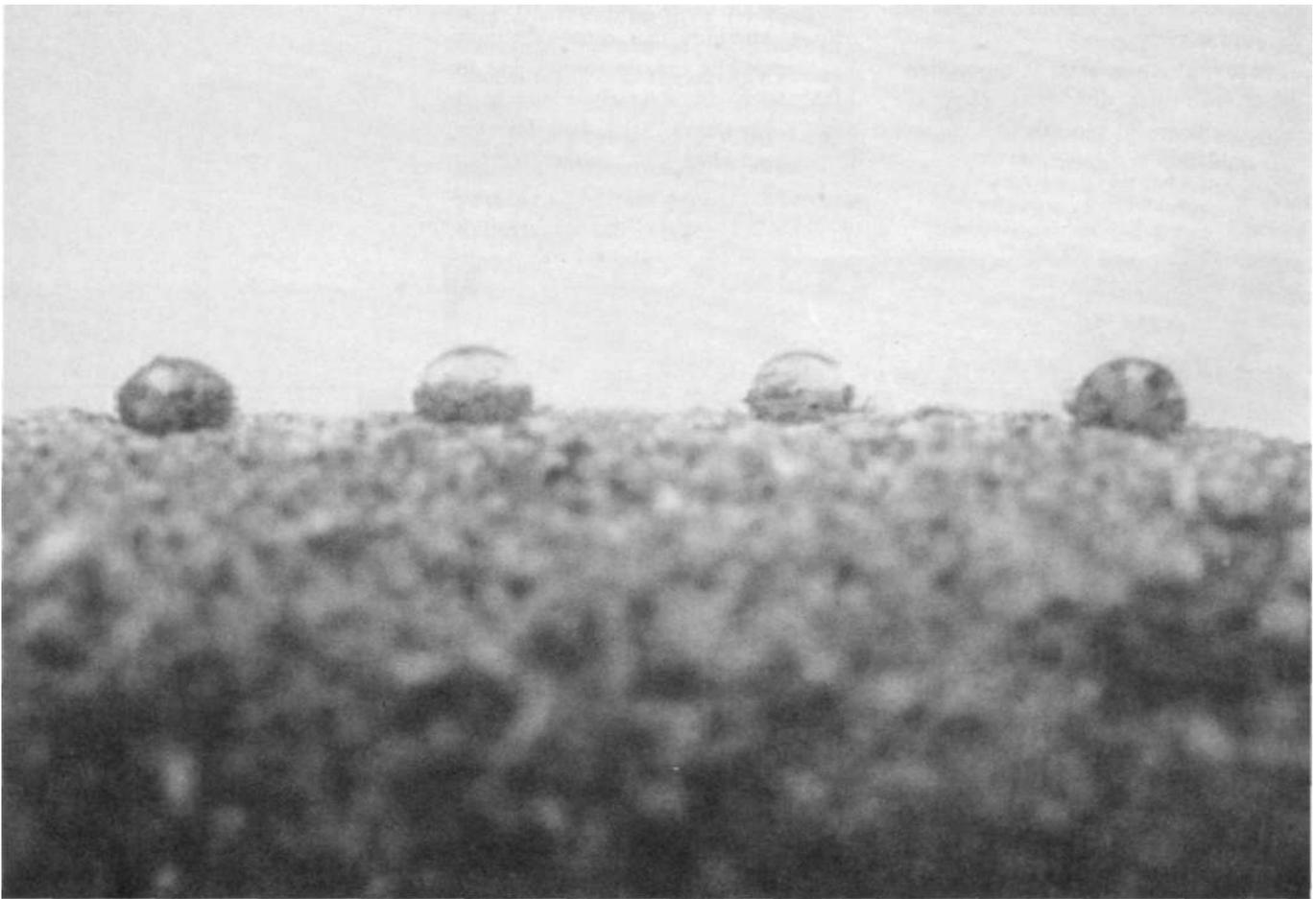
A core of a hydrophobic soil demonstrates its ability to resist water.
