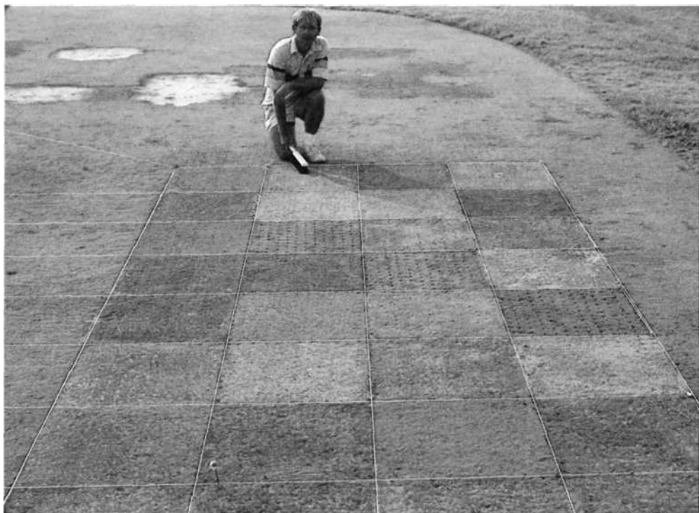
Here, a hydrophobic experimental Pennncross green was used as the test area for a coring/soil amendment study.
